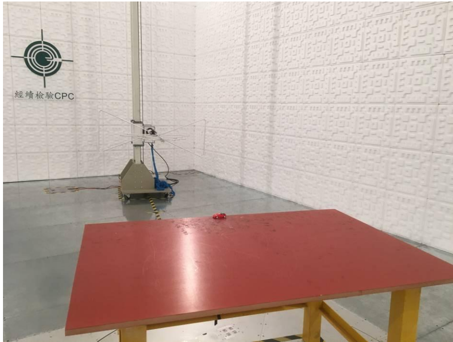
Set-up for radiated electromagnetic disturbances
